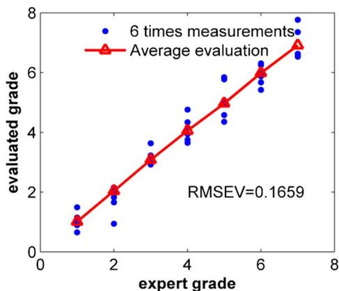
**Fig. 4.** Relationship between expert grades and evaluated grades of Shifeng Longjing tea with 2D fluorescence correlation spectroscopy based on intensity perturbation.
