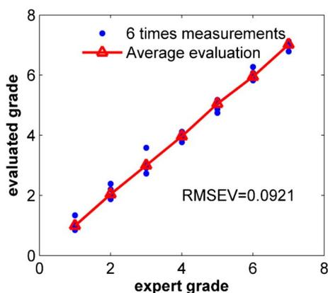
**Fig. 8.** Relationship between expert grades and evaluated grades of Shifeng Longjing tea with 2D fluorescence correlation spectroscopy based on excitation wavelength perturbation.
