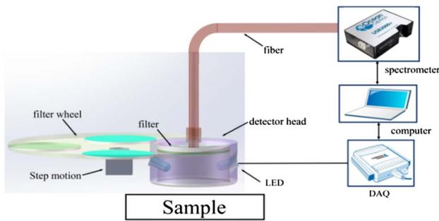
**Fig. 1.** Schematic of 2D fluorescence spectroscopy system based on LEDs.
