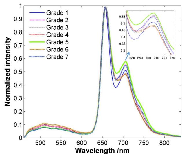
**Fig. 5.** Normalized fluorescence spectra for tea samples with seven different grades at the maximum excitation intensity. The inset is the magnified spectra around 710 nm.
